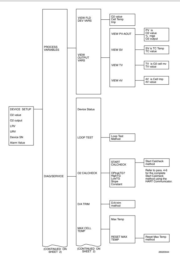
Figure 4-3. Menu Tree for HART/AMS on the Two-Wire In Situ Oxygen Analyzer (Sheet 1 of 3)
